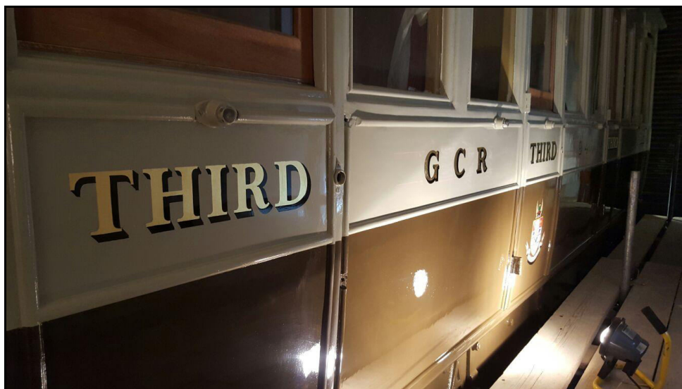
above: MS&L coach no.946 had not been moved out of the workshop following restoration at GCR(N) at Ruddington, however this close-up view clearly shows the museum standard quality of the paint-work and lining-out applied in October 2015. photo: GCR Rolling Stock Trust
